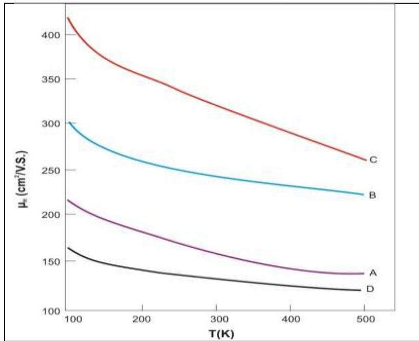
Fig. 3. Variation of Hall mobility ( $\mu_H$ ) with temperature. Curves A, B, C and D bear the same meaning as described in Fig. 1.
