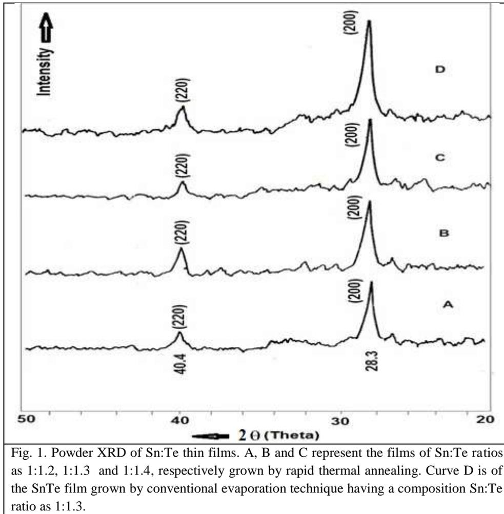
Fig. 1. Powder XRD of Sn:Te thin films. A, B and C represent the films of Sn:Te ratios as 1:1.2, 1:1.3 and 1:1.4, respectively grown by rapid thermal annealing. Curve D is of the SnTe film grown by conventional evaporation technique having a composition Sn:Te ratio as 1:1.3.
