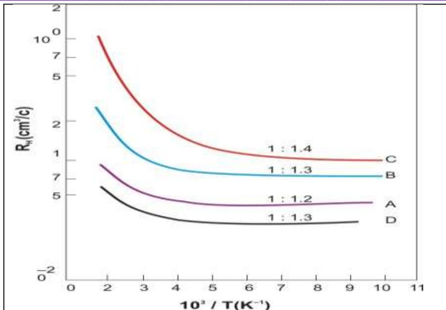
Fig. 2. Variation of Hall coefficient  $R_H$  with Temperature for SnTe films having different stoichiometric ratios. Curves A, B, C and D represent the same films as described in Fig. 1.
