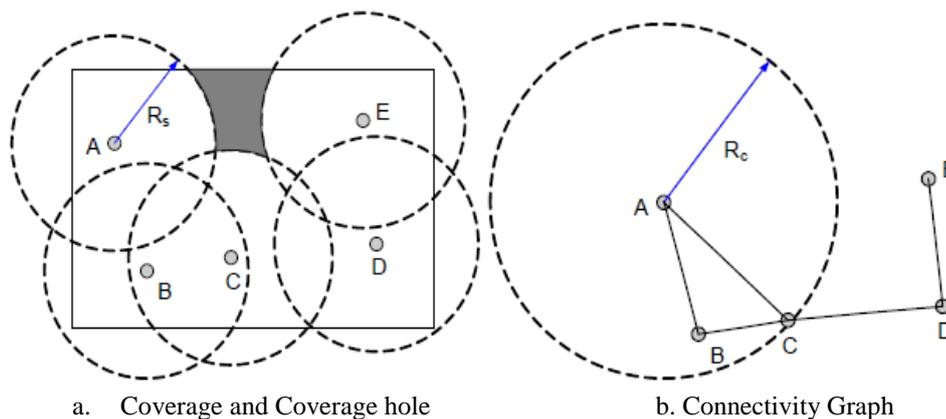
Figure 1.1: Illustrations of coverage and connectivity
