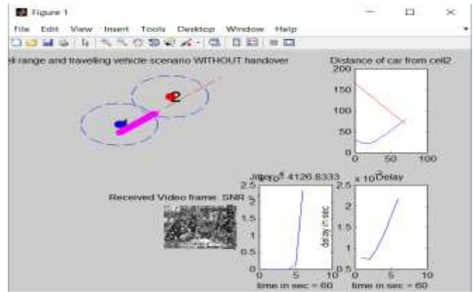
Fig.11 Received Video, Delay and Jitter Graph when Handover not executed
