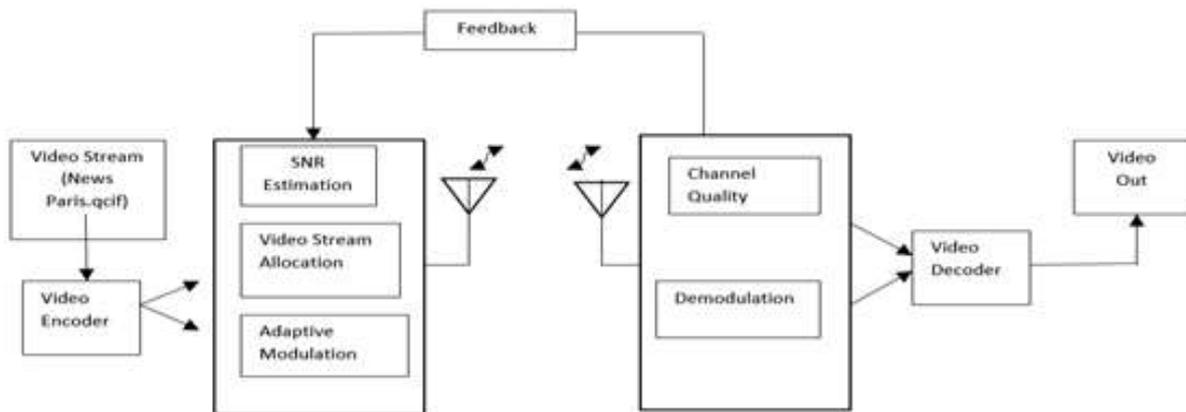
Fig.2 Architecture of proposed video streaming system
