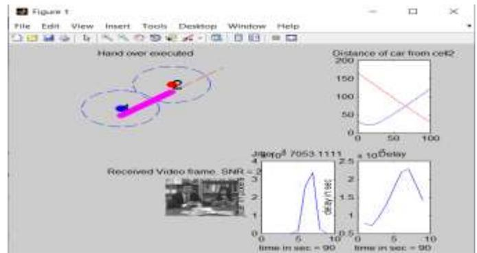
Fig.12 Received Video, Delay and Jitter Graph when Handover executed
