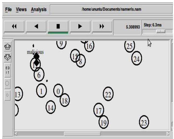
Figure 8 Dynamic malicious node in a network of 50 nodes and loss of packet
