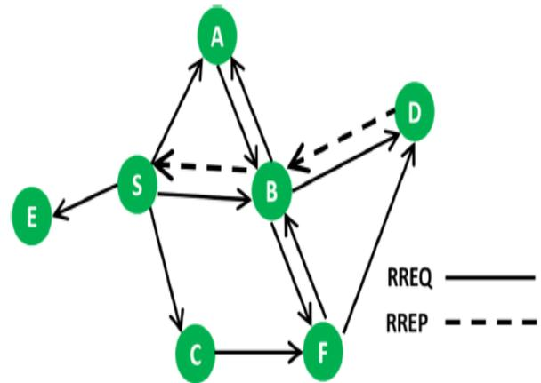
Figure 4 Route discovery process between nodes S and D
