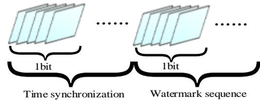
Figure 4. Time synchronization sequence and watermark sequence
