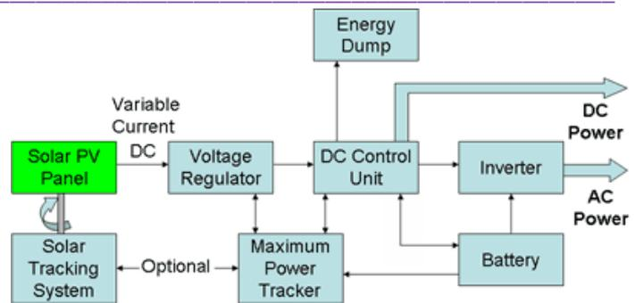
Photovoltaic Electric Power Generation
