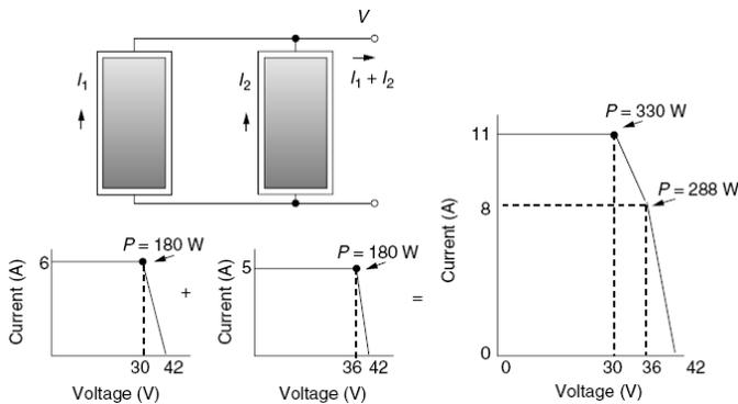
Each module is rated at 180 W, but the parallel combination yields only 330 W at the maximum power point.
