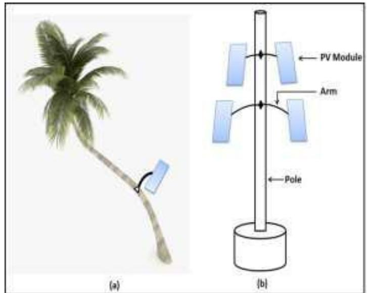
Fig. 4: Solar tree structure roof top model
