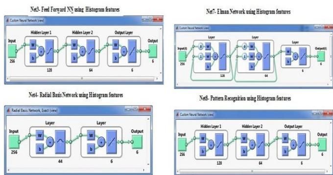
Figure6. Network structure of Feed Forward, Radial Basis, Elman and Pattern Recognition Neural Network
