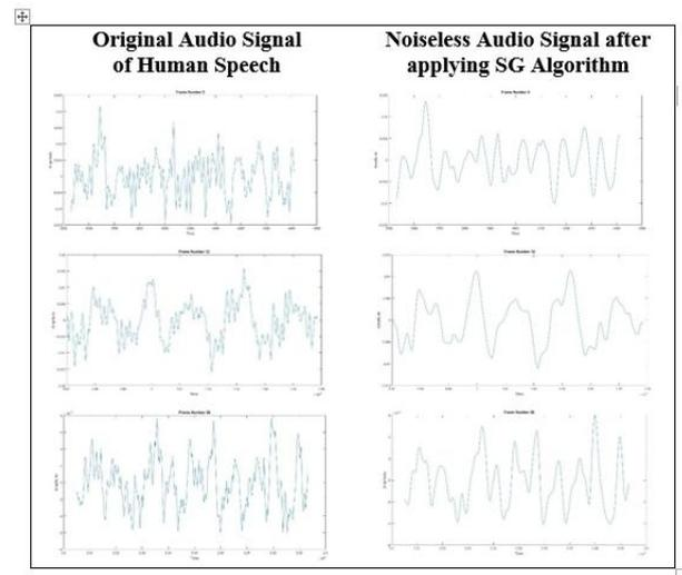
Figure 6. Input and Output Audio signals for Human Speech
