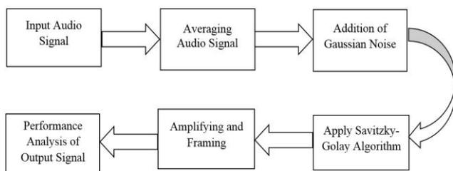
Figure 2. Block Diagram of Audio Noise Reduction System
