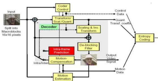
Fig:-1 blocks diagram of the H.264 encoder [6]
