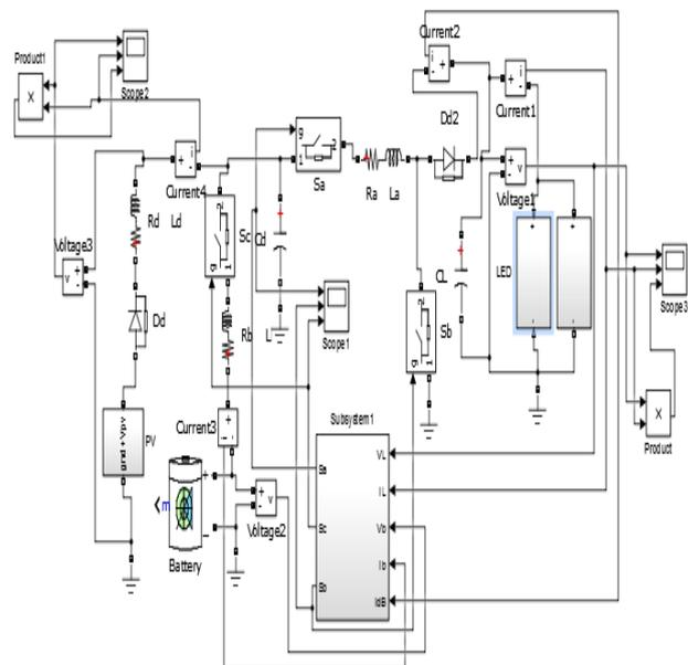
Figure 6: The general Matlab/Simulink model of PV array and Li-Ion battery powered LED lighting system.
