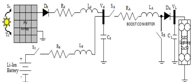
Figure 2. Test system PV and battery powered LED lighting system.
