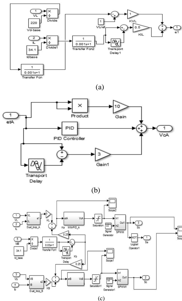
Figure (3): Multi loop error driven dual-loop regulator model (a), WM-PID controller model (b), Dual loop, dual regulator hybrid controller model (c).
