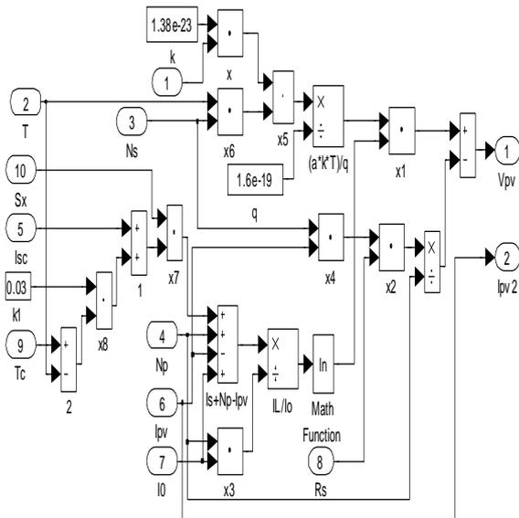
Figure 4. PV Array Matlab/Simulink functional model.
