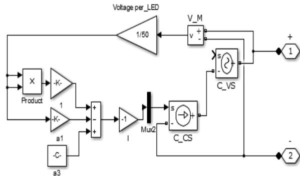
Figure 5. Matlab/Simulink model for 50 fixtures LED
