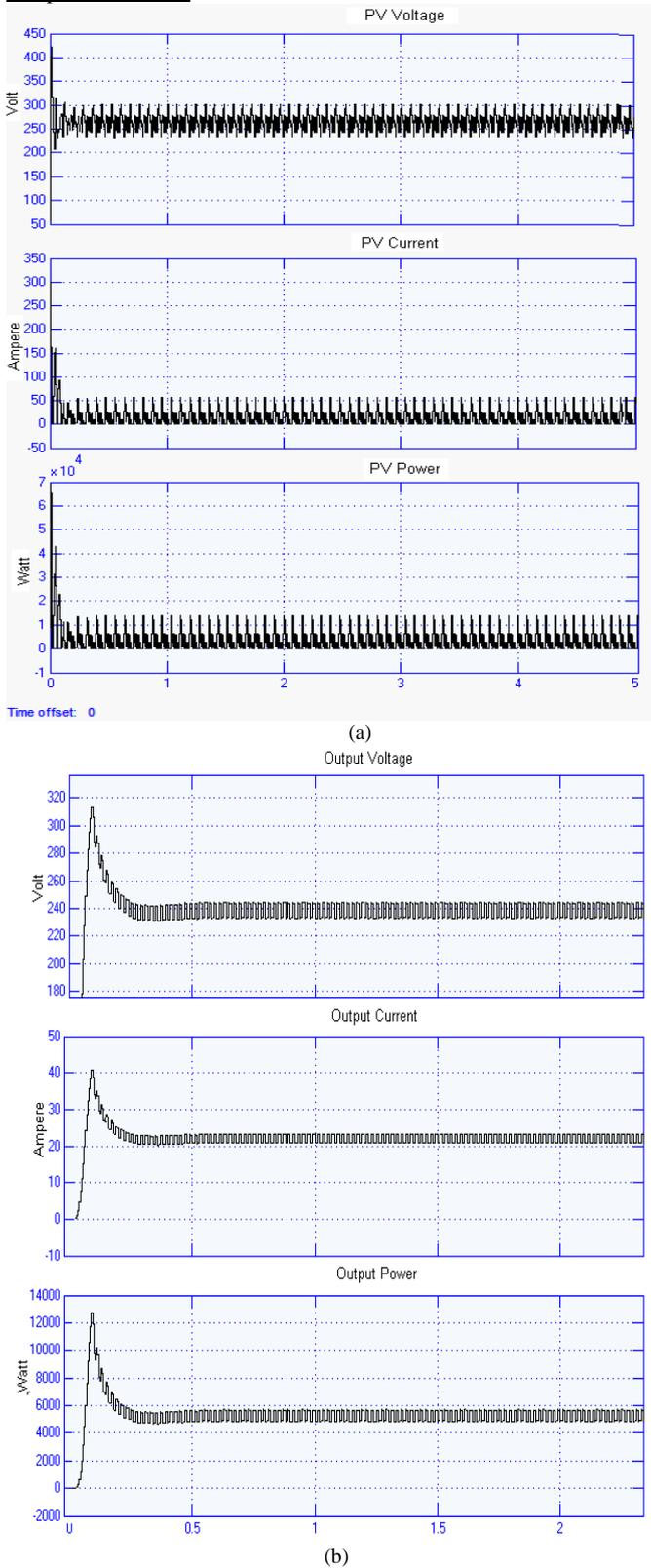
Figure 7. (a) PV voltage, current and power, (b) output voltage current and power simulation results for SOC 90%.
