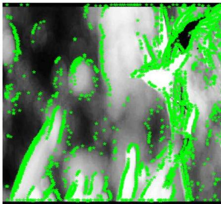
Fig. 4 Feature extraction obtained by scale invariant feature transform
