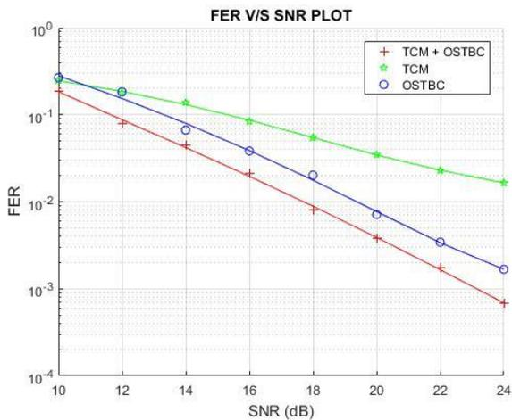
Fig. 5: Simulation result for 2x1 TCM+OSTBC, TCM and OSTBC (Rayleigh Channel)
