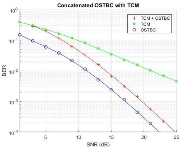
Fig. 4: Simulation result for 2x1 TCM+OSTBC, TCM, OSTBC (Rayleigh Channel)
