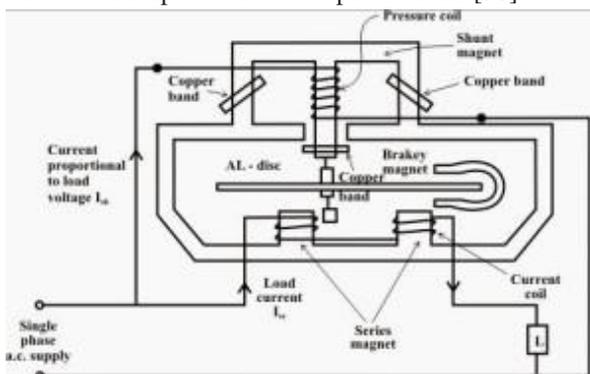
Figure 3 Working of induction type energy meter [30]
