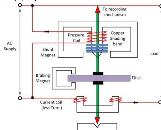
Figure 1: Energy Meter connection diagram [31]
