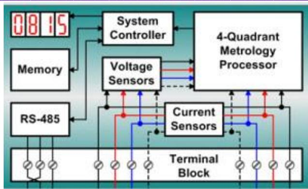
Figure 5 Digital Electronic Energy Meters [30]
