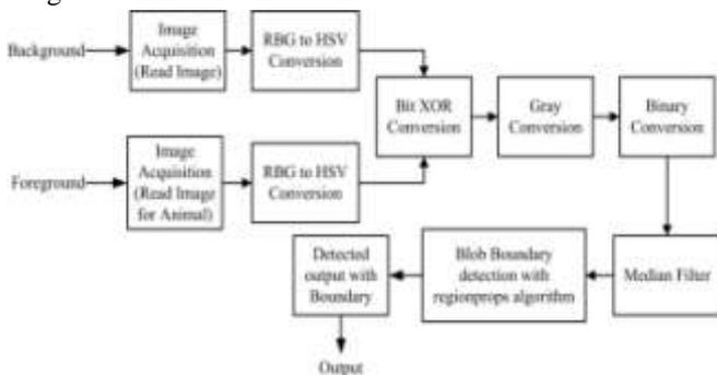
Figure 3.1: Block Diagram of animal detection using background subtraction
