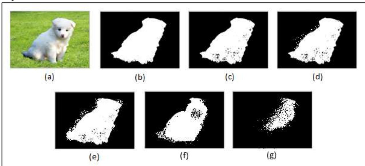
Figure 4.9: Visual comparison on background subtraction a) sample frame b) ground truth c) proposed method d) Method\_2 e) Method\_1 f) GMM method g) FD method
