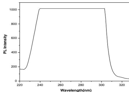
Figure-3.4.1 Excitation spectrum of Eu(1.5%) and Tb(2%) doped  $Y_2SiO_5$  phosphor monitored under 615nm.
