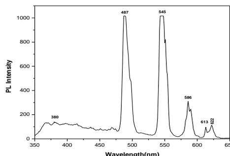
Figure-3.4.2 Emission spectrum of Eu(1.5%),Tb(2%) doped  $Y_2SiO_5$  phosphor under the excitation of 254nm.
