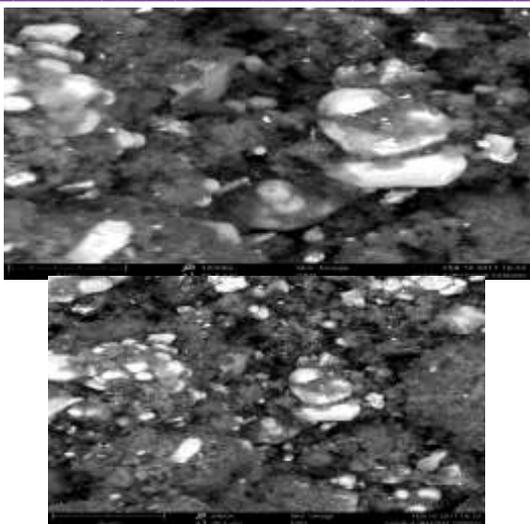
Fig.3.2.SEM Image of Tb(2%),Eu(1.5%) doped  $Y_2SiO_5$
